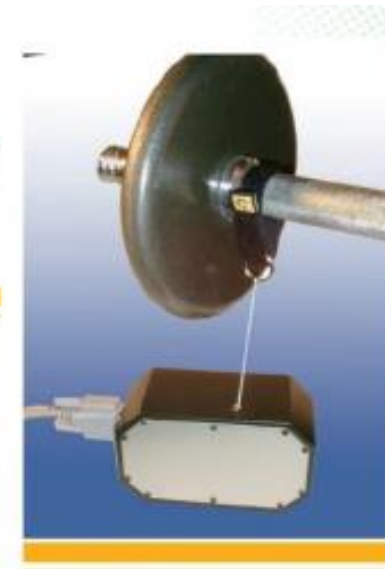
Figura 27. Muscled power linear encoder Fuente: Extracto de http://www.muscle-europe.it/products/ibferrero-27/muscle-lab-07ferrero-3646-accessories
